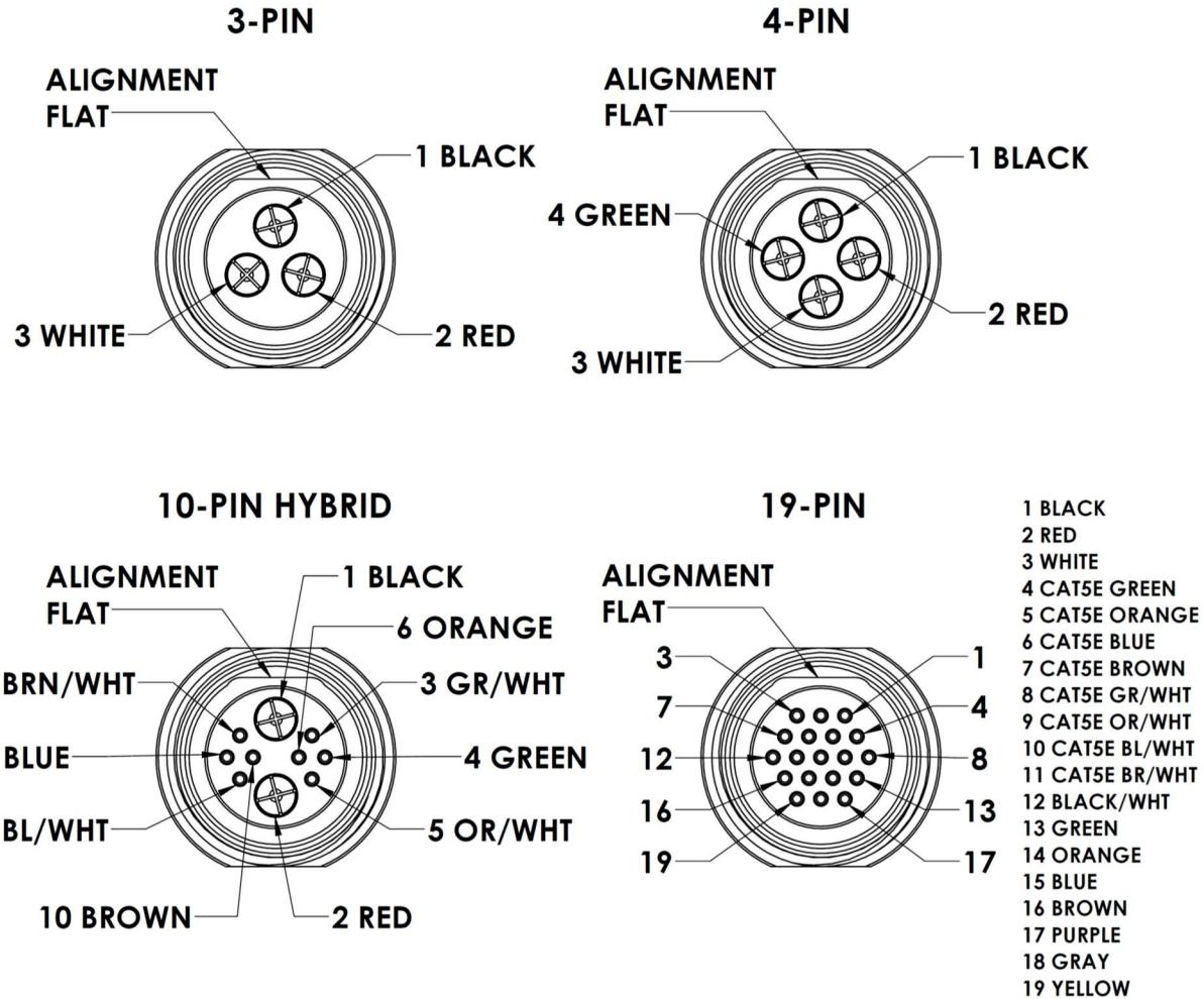
Cable connector pinouts (looking at mating face of connector)
