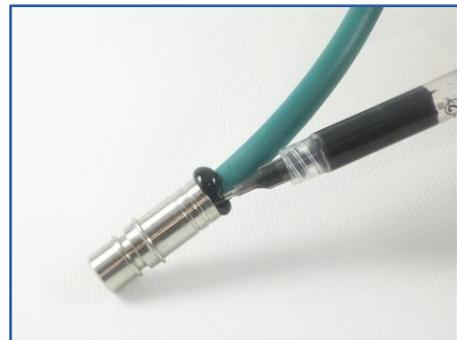
17. Clean off the excess epoxy with a paper towel and acetone or alcohol.
