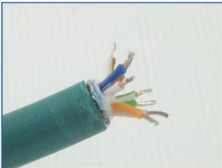
5. Insert the wires into the sockets on the Connector Insert and solder them in place. It is very important to make a clean solder joint with minimal solder outside the joint – excess solder can cause shorts between the wires or between a wire and the Connector Shell. Double-check that each wire is soldered to the correct socket (the pinout will depend on the particular application).
