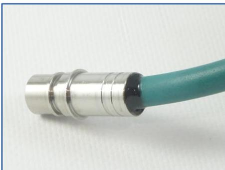
18. Allow the epoxy to cure fully without disturbing the assembly. When fully cured, check for electrical shorts one more time with a multimeter.
