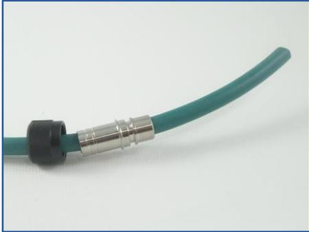
4. Strip the last 1-2 cm of cable jacket off your cable. Trim the wires as close to the end of the cable jacket as possible, while still allowing enough room to solder them to the Connector Insert. Strip the last 5-6 mm of insulation off the wires. Make sure the strands of wire are tightly wound and that there are no loose or protruding strands which could cause an electrical short. Tin the ends of the wires with solder to prevent the wire strands from fraying.
